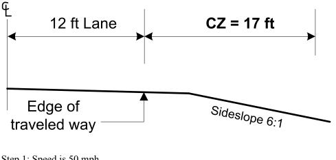
Step 1: Speed is 50 mph Step 2: Traffic is 320 ADT Step 3: Sideslope is 6H:1V Step 4: Read 17 feet directly from table **Control Zone = 17 feet**
