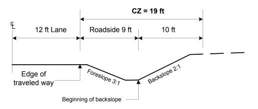
Step 1: Roadside width is 9 feet Step 2: 9 feet plus 10 feet = 19 feet **Control Zone = 19 feet**
