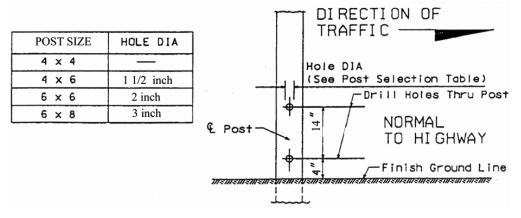
**Note:** Posts that are larger than 6" x 8" require barrier protection when located within the Control Zone. (See the *Standard Plans* for further guidance.)
