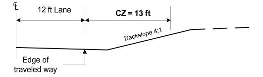
Step 1: Speed is 45 mph Step 2: Traffic is 1900 ADT Step 3: Backslope is 4H:1V Step 4: Read 13 feet directly from table **Control Zone = 13 feet**
