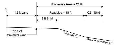
Step 1: Speed <u>is</u> 40 mph Step 2: Traffic <u>is</u> 3000 ADT Step 3: Existing ground sideslope <u>is</u> 6H:1V Step 4: Read from table, CZ is 16 feet Step 5: Roadside width <u>is</u> 18 feet Step 6: Shoulder width <u>is</u> 8 feet Step 7: (18 feet) + (16 feet - 8 feet shld) = 26 feet **Control Zone = 26 feet Note:** For positive (+) ground sideslopes, use Condition 3 or 4.
