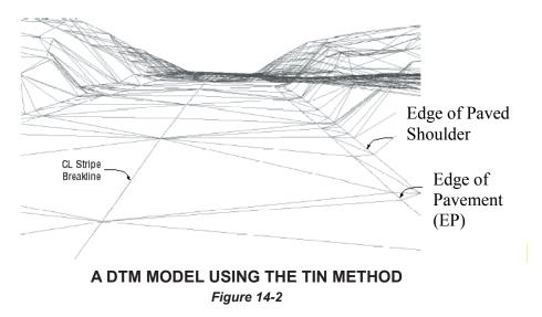
Breaklines define the points where slopes change in grade (the intersection of two planes). Examples of Breaklines are the crown of pavement, edge of pavement, edge of shoulder, flow line, top of curb, back of sidewalk, toe of slope, top of cut, and top of bank. Breaklines within existing highway rights of way are clearly defined, while breaklines on natural ground are more difficult to determine.
