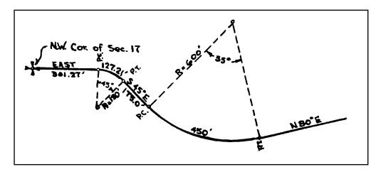
A compound curve is one in which the radius of the curve is changed somewhere along the arc without the intervention of a tangent course.
