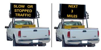
Truck-mounted PCMS displays two messages for 2 second each of a work zone queue ahead. "NEXT # MILES" will be rounded up to the nearest whole mile. **Source:** Modified from Trafcon
