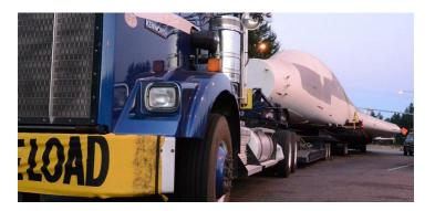
Superload truck freight example; Boeing B1 bomber 131 feet long, 29+ feet wide, and 15 feet high. *Source:* WSDOT
