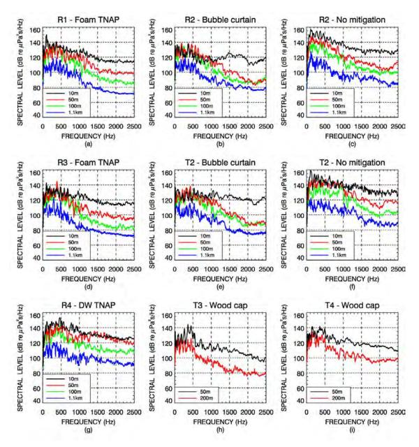
Figure 7: Plots of mean spectral energy levels as a function of range for steel and concrete piles measured during the Test Pile project.
