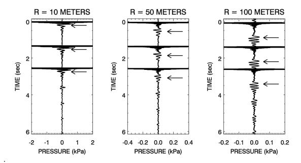
Figure 9: Waveform plots showing seismic interface waves (Scholte waves) generated during the driving of pile T2 at 10 meters, 50 meters and 100 meters distance. The Scholte waves are indicated by arrows on the plots. Note that the waveforms have been amplified to emphasize the interface waves.
