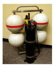
Figure 4: Photograph of a JASCO autonomous Ocean Bottom Hydrophone (OBH) recorder system. The OBH stands approximately 1 meter tall.
