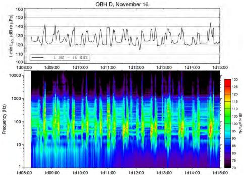
Figure 10: Continuous background measurements at station "D" (1.1 km) for 16 November 2006. Top plot shows broadband 1-minute average sound levels versus time. Bottom plot shows spectral power levels versus time. Times are given in hours from midnight.
