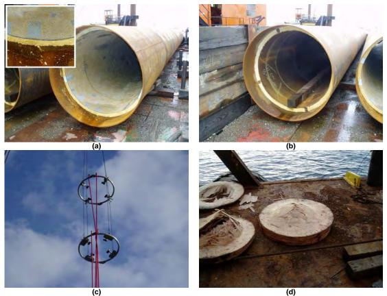
Figure 2: Photographs of attenuation methods tested during the current study: (a) Foam-walled TNAP (inset shows detail of foam); (b) double-walled TNAP; (c) bubble curtain; (d) wood pile caps.
