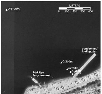
Figure 3: USGS aerial photomosaic of study site with annotations showing OBH deployment locations (A, B, C and D) and pile driving site.
