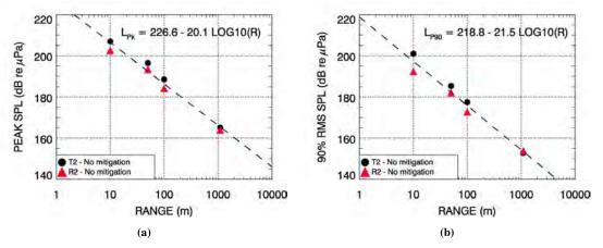
Figure 8: Acoustic propagation loss versus range for (a) peak and (b) 90% *rms* level data fit by least-squares analysis to pile T2 data. Dashed line indicates the best fit to the data; the equation with the fit parameters is shown in the plot annotation.
