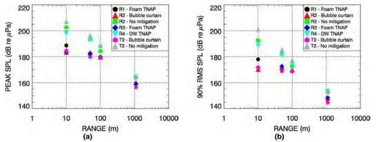
Figure 5: Average (a) peak and (b) 90% RMS sound pressure levels versus range for the steel piles (R1-R4 and T2) measured on 16 November 2006.
