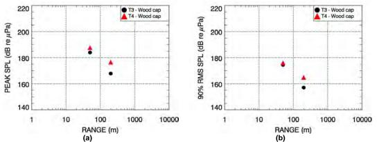
Figure 6: Average (a) peak and (b) 90% RMS sound pressure levels versus range for the concrete piles (T3 and T4) measured on 5 December 2006.
