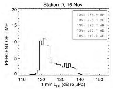
Figure 11: Histogram of 1 minute  $L_{eq}$  background levels for 7 hours at station "D" on 16 November 2006. Percentiles ambient noise levels from the histogram are shown in the plot annotation. Note that the N% noise level is defined as the  $L_{eq}$  that was exceeded during N% of the total recording time.
