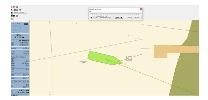
08:13:54 PDT stern handle moved from position 8 ahead to position 10 astern.
