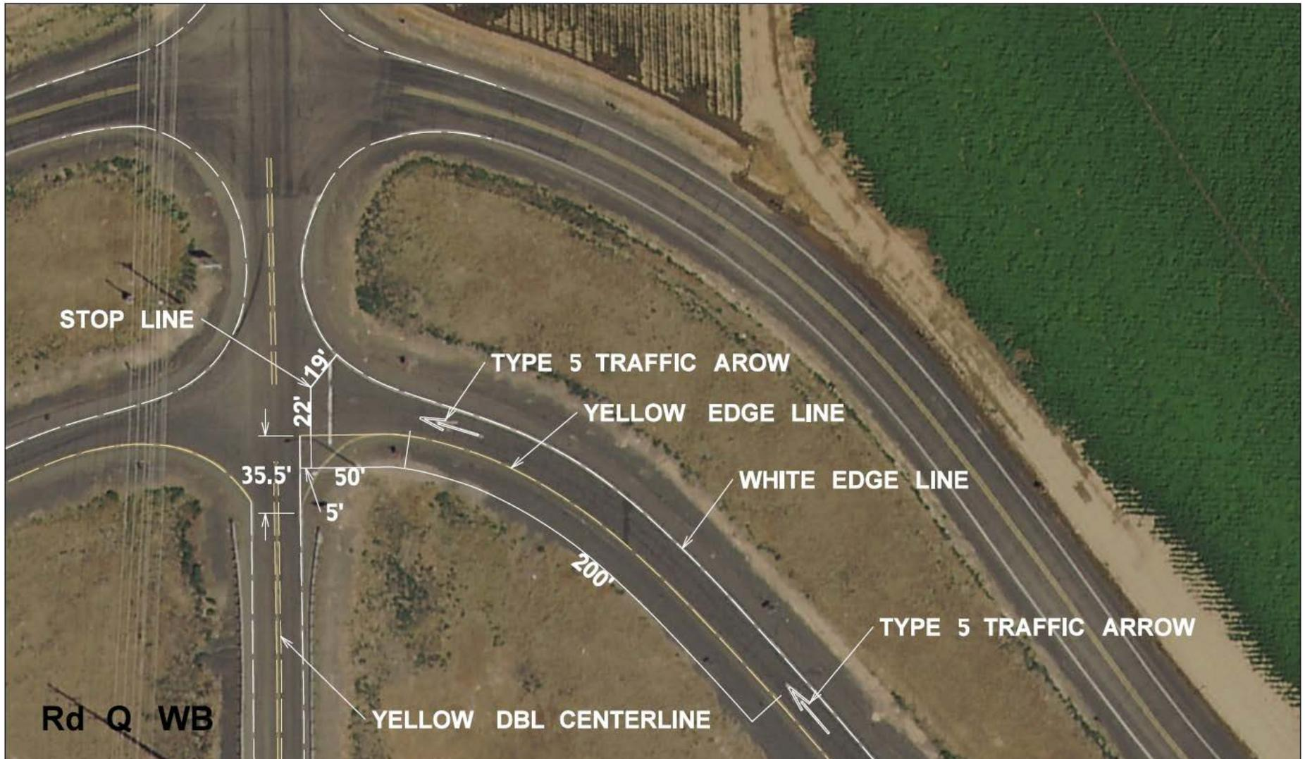
North Central Region Figure 7 - Interstate 90 Westbound Road Q - Improved Pavement Markings Plan, including updating directional arrows, centerline and edge line pavement markings
