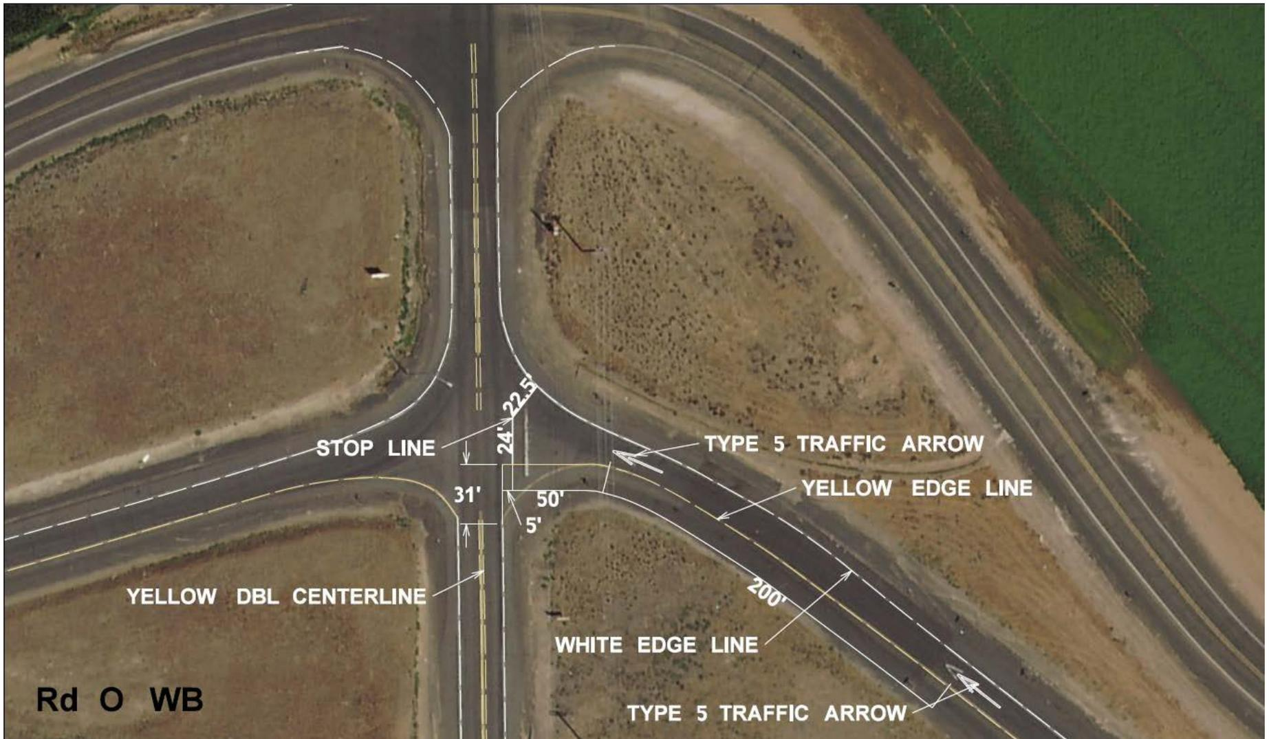
North Central Region Figure 3 - Interstate 90 Westbound Road O - Improved Pavement Markings Plan, including updating directional arrows, centerline and edge line pavement markings
