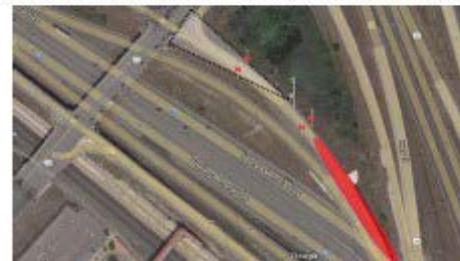
Carmanah Technologies Corp. Wrong-Way Driving Countermeasure Proposal, an example of the 3 detection zones that the equipment uses
