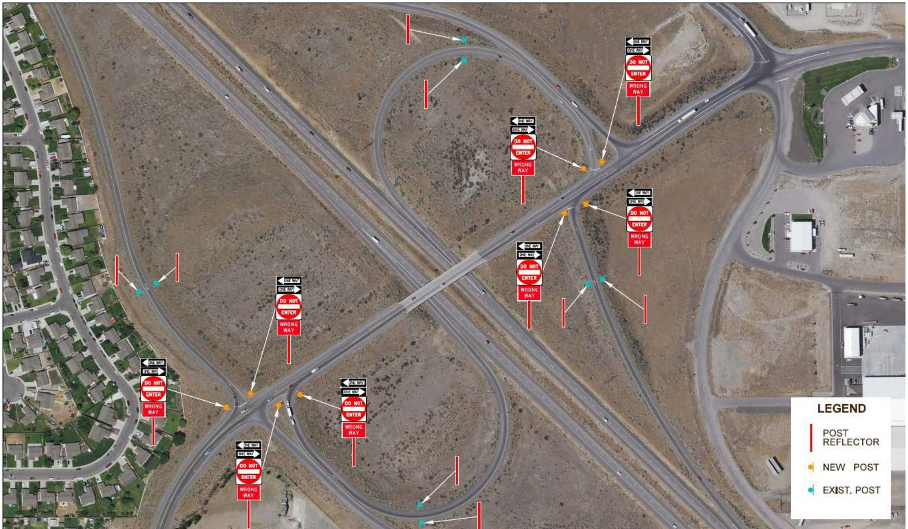
South Central Region Figure 2 - US Highway 12 Interchange at Lewis Street - Signing and Pavement Marking Improvement Plan
