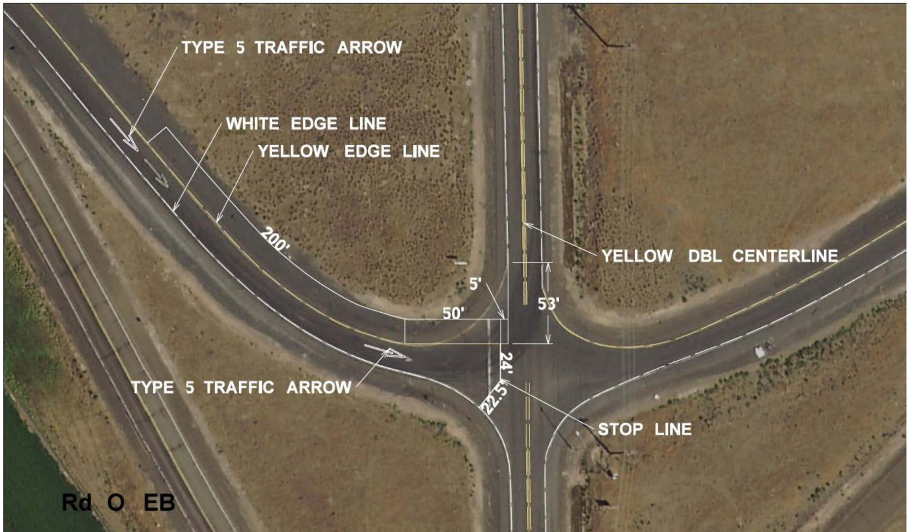
North Central Region Figure 1 - Interstate 90 Eastbound Road O - Improved Pavement Markings Plan, including updating directional arrows, centerline and edge line pavement markings
