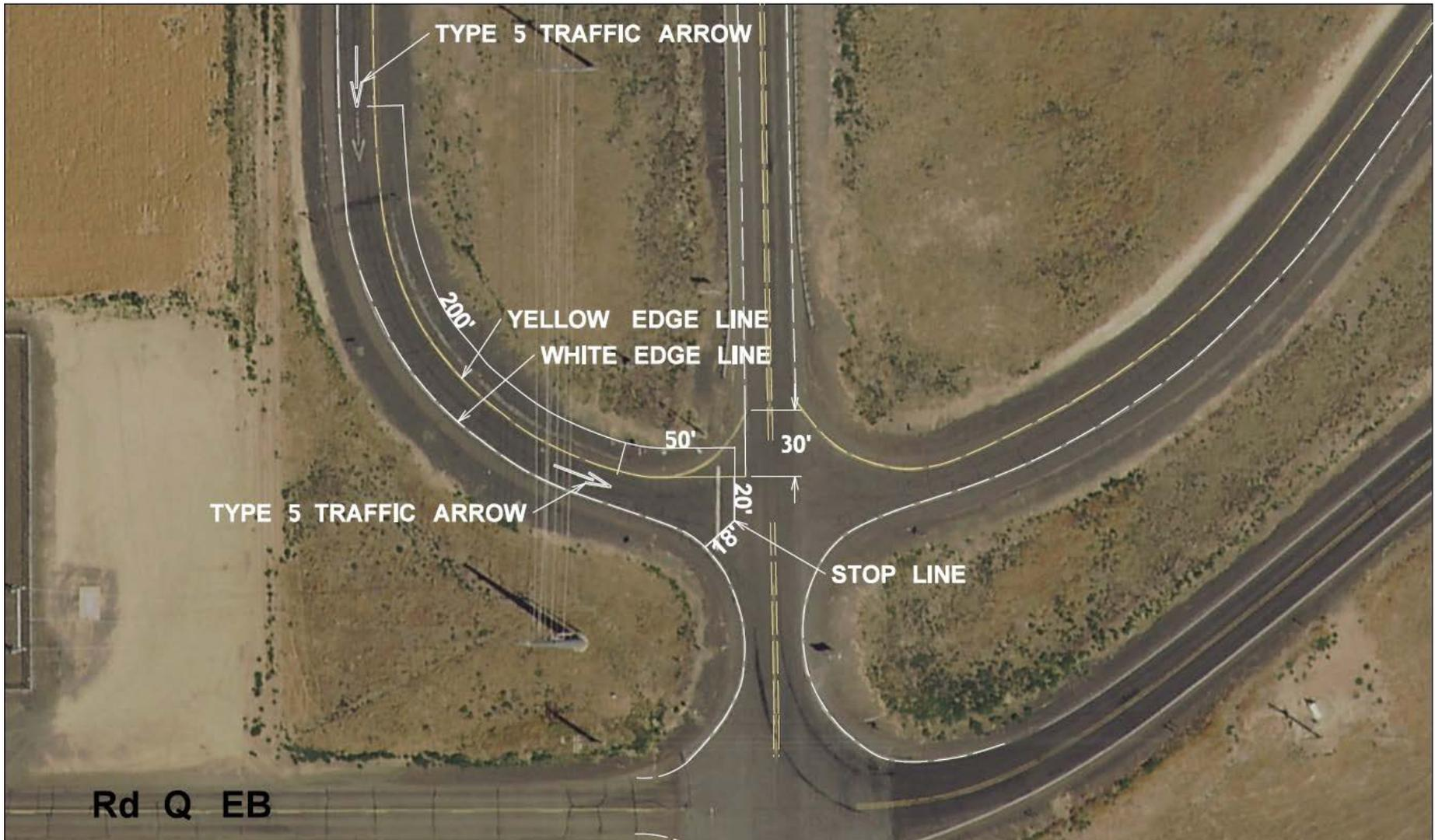
North Central Region Figure 5 - Interstate 90 Eastbound Road Q - Improved Pavement Markings Plan, including updating directional arrows, centerline and edge line pavement markings
