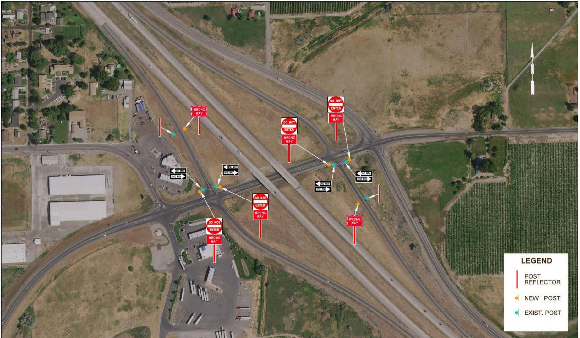
South Central Region Figure 3 - Interstate 82 Interchange at Exit 58 - Signing and Pavement Marking Improvement Plan
